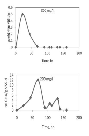
Figure 2. The trend of biogas production in different oxytetracycline concentration
